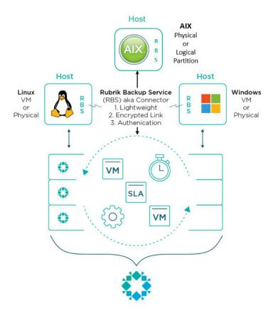
The RBS software can only be used with the Rubrik cluster from which the software is obtained. Each Rubrik cluster generates a copy of the RBS software that includes authentication information specific to that Rubrik cluster. This method ensures that the Rubrik cluster and a hosted deployment of the RBS can reliably authenticate each other. As an additional security measure, all communication between Rubrik and RBS is encrypted.
