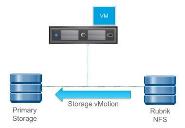
Ultimately, Rubrik serves as a storage endpoint to recover as many vSphere VMs as needed, thus eliminating the complexity and time wasted in transferring data back into the production system. This functionality provides a near-zero recovery time and restores user access near instantly.
