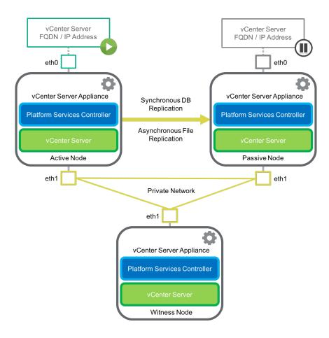
When vCenter HA configuration is complete, only the Active node has an active management interface (public IP). The three nodes communicate over a private network called vCenter HA network that is set up as part of configuration. The Active node and the Passive node are continuously replicating data. This data includes:
