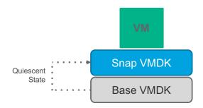
To help minimize the time that a VM is quiescent, the Rubrik cluster maintains multiple concurrent connections with a vSphere environment and opens five threads for each ESXi host in that environment.
