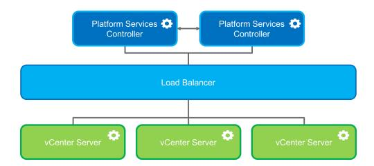
The vCenter Server nodes are connected to the load balancer. When a Platform Services Controller instance stops responding, the load balancer automatically repoints the vCenter Servers registered the unavailable Platform Services Controller to other functional Platform Services Controller node without downtime.
