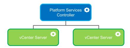
It is recommended to protect each vCenter Server Appliance node and at least one Platform Services Controller (if in the same SSO domain). If there are multiple SSO domains, then a minimum of one Platform Services Controller should be protected in each SSO domain.
