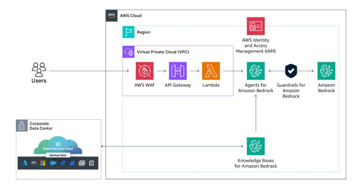
Programmatic access is provided to Amazon Bedrock to seamlessly integrate the Rubrik enterprise data sources in the AI architecture, which then can be leveraged for retrieval-augmented generation.
