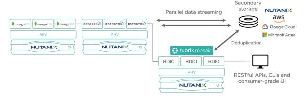
Rubrik Mosaic is a software platform that can be deployed in any form factor, such as VMs on-premises, software instances in any cloud provider, or as Docker containers. Deployed as a 3-node or 5-node cluster, Rubrik Mosaic does not store your data but sends data directly from the source clusters to the backup target, such as Nutanix Acropolis VM storage, NFS, AWS S3, Google Cloud, Microsoft Azure or S3 compatible private object storage (e.g. EMC ECS, Cloudian, and Scality).
